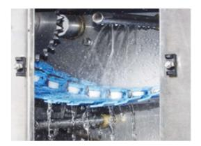
• The cabinet has a standard built in belt wash. A wash tank contains wash arms located above and below the belt to thoroughly spray the belt with water.
